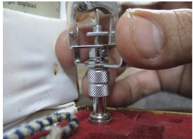
Fig. 2: Checking Schiotz tonometer for zero error
