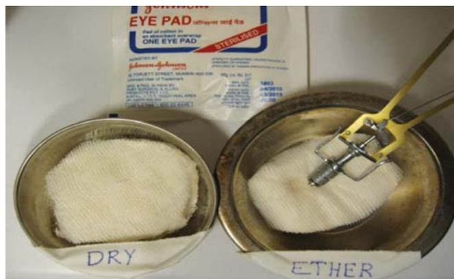
Fig. 4: Cleaning of Schiøtz tonometer
