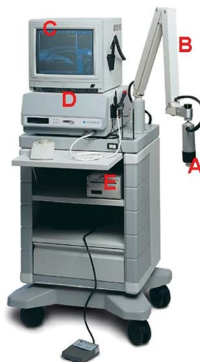
Fig. 1: The current UBM—P45 workstation (Paradigm Medical Industries, UT, USA). A: Ultrasound transducer and probe; B: Articulated arm; C: Computer monitor; D: Main processing unit; E: Printer
